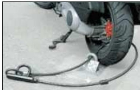
Fig 58: Secure ground level anchor point.
