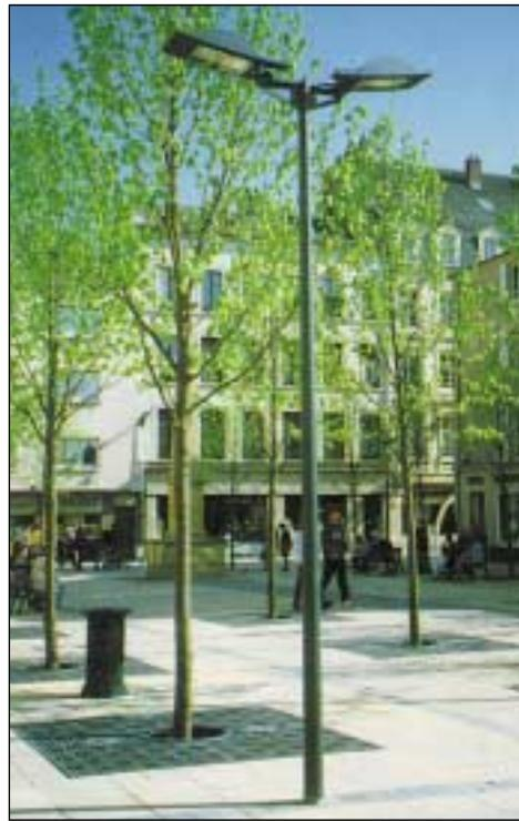
Fig 31: Trees with no foliage below 2m maintaining visibility. (External works, 11th Edition p.485)
