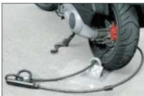
Fig 58: Secure ground level anchor point. Source: Department for Transport.
